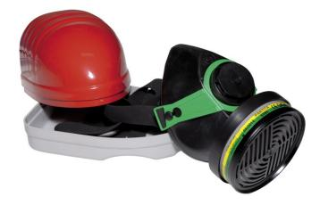
**Filter type emergency** respirator for escape from buildings and industrial areas in case of accidental pollution by toxic gases or vapours. Type A-B-E-K, lasts at least 15 min. according to the DIN 58647-7. It doesn't give protection from dusts, fumes or carbon monoxide. It is not therefore suitable in case of fire.
