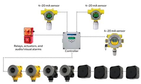
Up to eight digital sensors via Modbus RS-485 communication from the Sensepoint XCL and XRL sensors
