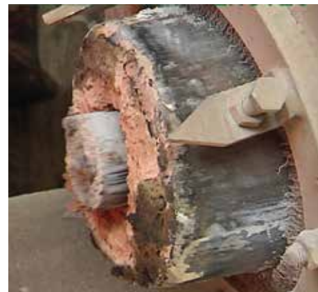
Fig. Automated plunger keeps the flue gas entrance free of blockages.
