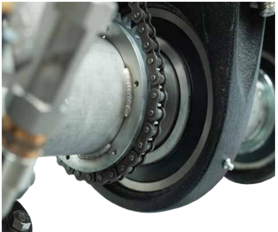
Fig. The powerful probe rotation device prevents thermal bending and sticking
