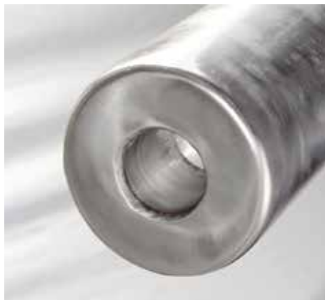
Fig. Automated plunger keeps the flue gas entrance free of blockages.
